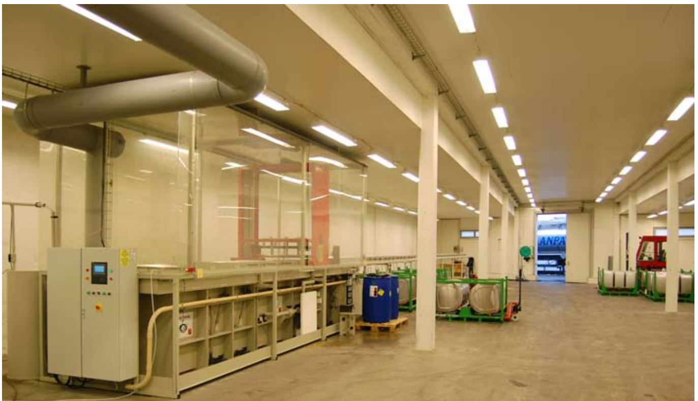
The 30-metre long, specially built, pickling line at Avesta Finishing Chemicals.
