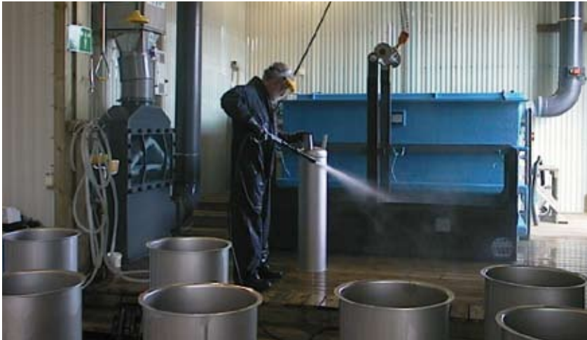
Figure 11: High-pressure rinsing after pickling.
