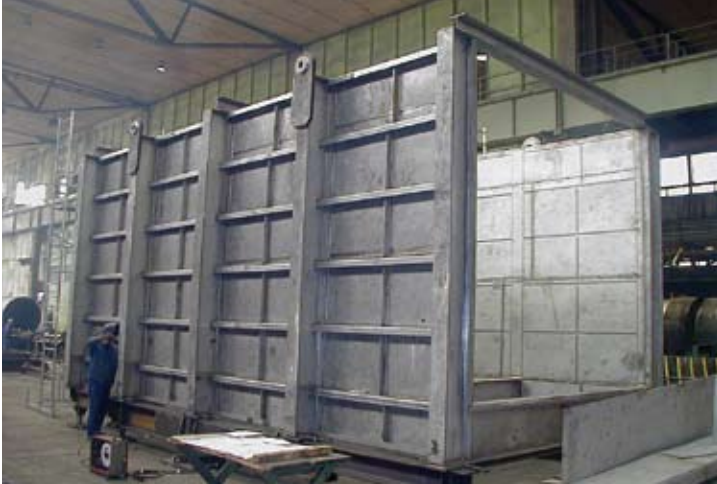
Figure 8: Typical stainless steel object ready for spray pickling.
