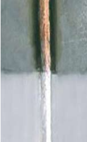
Figure 1: Before and after pickling
