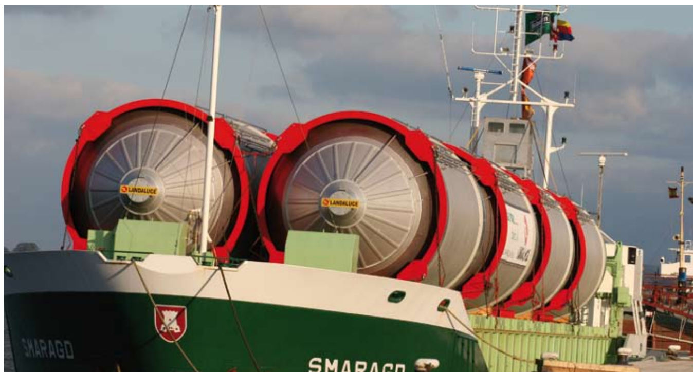
Figure 10: Stainless steel beer tanks ready for shipping after complete cleaning using Avesta products (photo courtesy of Landaluce)
